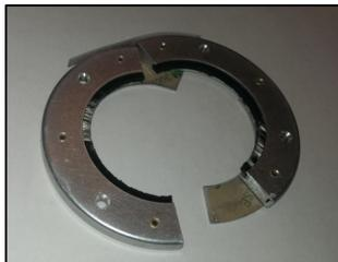
Figure 9 Shaft grounding brush
