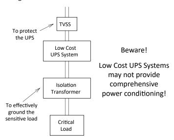
Most UPS systems are supplied with a limited battery capacity, typically capable of supplying 10-15 minutes of emergency power. If longer hold-up time is required, remember to factor in the costs of additional batteries.
