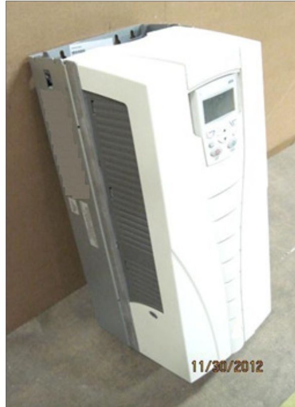
Figure 5 20 HP AFE drive
