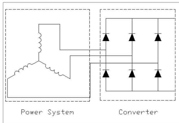
Figure 2 6-pulse power system and converter
