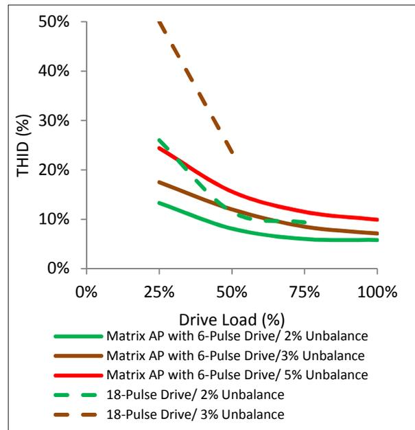
Figure 11 Matrix AP with 6-pulse drive and 18-pulse THID with system voltage imbalance
