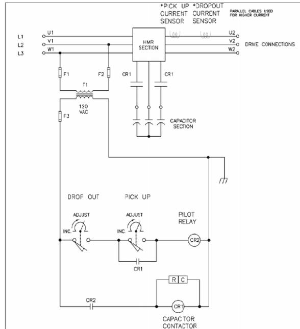
Figure 13 MTE Option -009 capacitor disconnect option schematic
