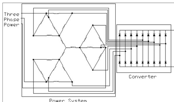
Figure 4 Nine phase power system and 18-pulse converter
