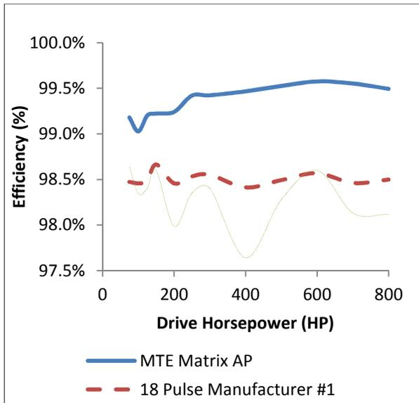
Figure 9 Percent efficiency of the added 18-pulse components and Matrix AP
