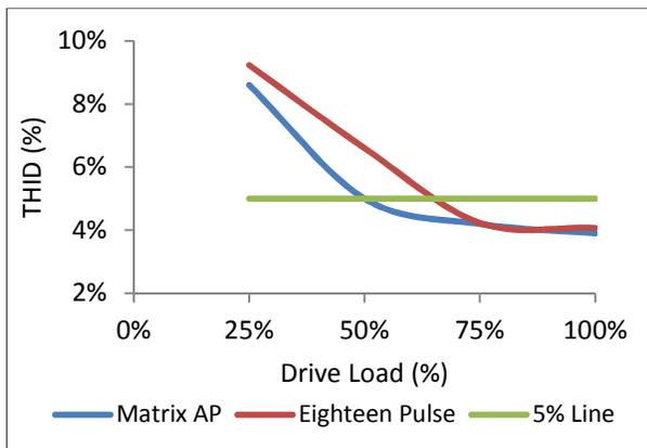
Figure 10 Matrix AP with 6-pulse and 18-pulse THID versus Load
