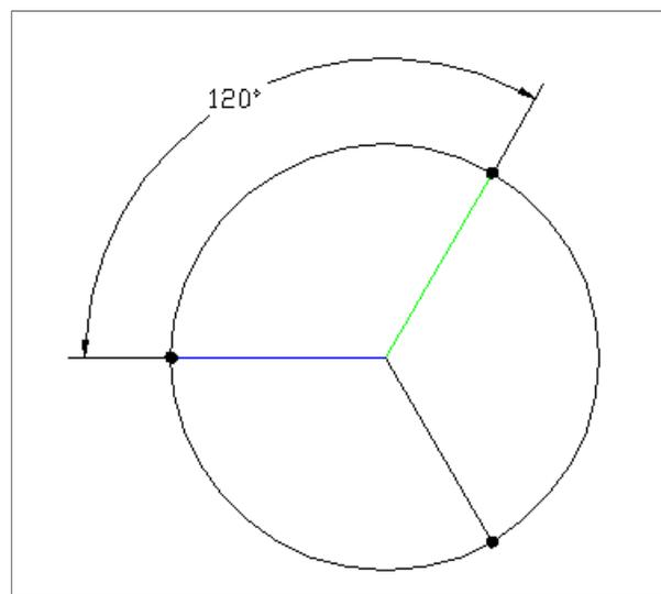
Figure 3 Three phase power system voltage vector representation
