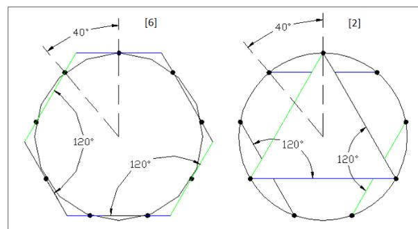
Figure 5 18-pulse vector representations of transformer windings
