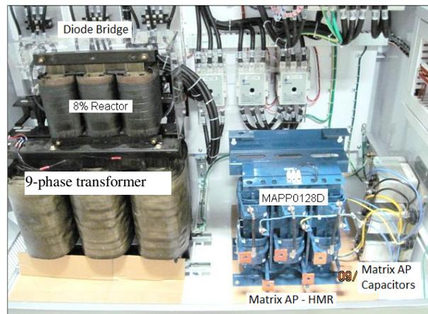
Figure 14 100 HP 18-pulse transformer and MAPP0128D
