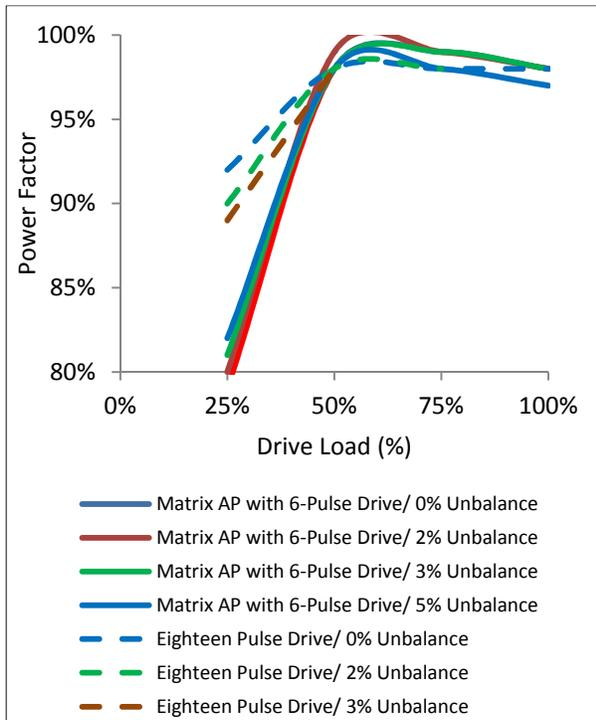
Figure 12 Power factor versus load
