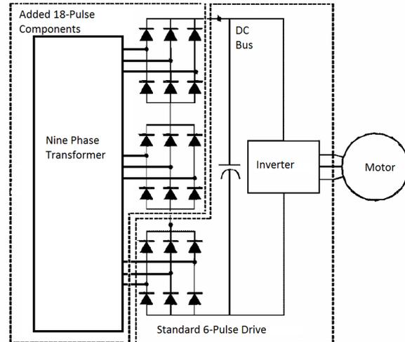
Figure 7 6-pulse drive conversion to 18-pulse
